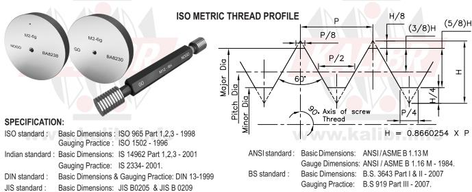
ANSI & BS standards use unilateral Tolerances for gauges. These gauges are manufactured only against specific customer order. We require Minimum Ordering quantity for these.
